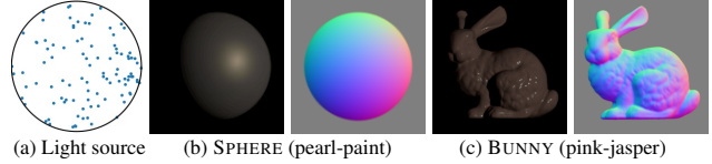
Figure 3. (a) Lighting distribution of MERL Test dataset. The light direction is visualized by mapping a 3-d vector [x, y, z] to a point [x, y] . (b) and (c) show a sample image and ground-truth normal for SPHERE and BUNNY, respectively.
