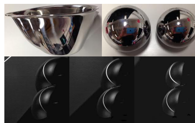
Fig. 18. Sauce boat and two spheres in real data experiments. Top row: sauce boat and two spheres in real experiments. Bottom row: a sweeping line is reflected by two spheres under three distinct positions of the LCD monitor while the camera and mirror surfaces are stationary.
