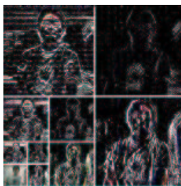
Fig. 2. Image pyramid formed from discrete wavelet transform. At each transform step, 4 components are extracted. The component at the top left corner of the result image is W_\psi^V(x, y) , that on the top right corner is W_\psi^D(x, y) , that on the bottom right corner is W_\psi^H(x, y) and that on the bottom left corner is W_\phi(x, y) . Transformation is done recursively on W_\phi(x, y) according to the wavelet theory.
