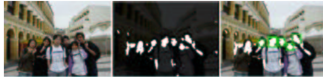
Fig. 5. This figure shows the face detection result on the image with multiple faces. The left image is the input image. The middle one shows the resultant binary image of the skin detection. The right image shows skin regions detected (in white color) and faces detected (in green box).
