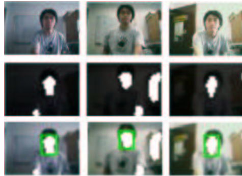
Fig. 4. Each column in this figure shows the face detection result of the input image at first row. The input images show variation in illumination. Second row shows the resultant binary image of the skin detection. Third row shows skin regions detected (in white color) and the face detected (in green box).
