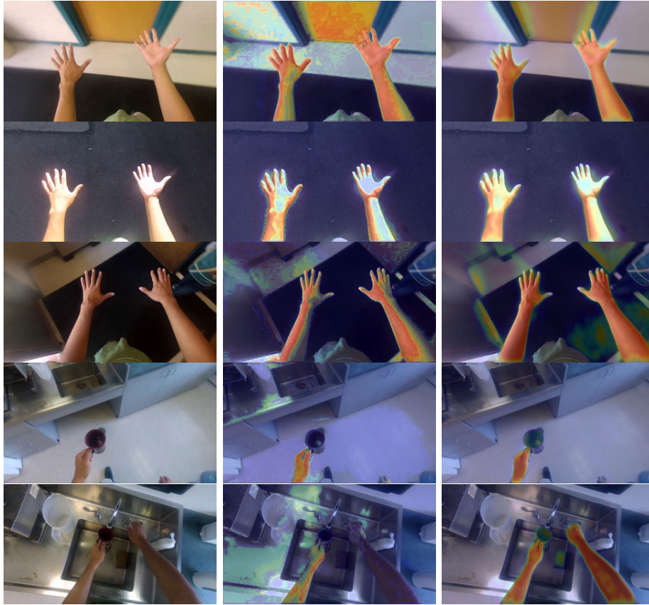
Figure 8: Sample images of EDSH data set: (left column) original images, (second column) results of Li and Kitani’s Method [5], and (last column) our results. From top to bottom: confusion with the door in EDSH1; shadow on the hand in outdoor in EDSH2; poor light condition in EDSH2; motion blur in EDSH-Kitchen; confusion with sink in EDSH-Kitchen. Best viewed digitally at high zoom.
