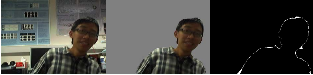
Figure 10. Segmentation with cluttered background. Left: current frame. Middle: segmentation result of the proposed method. Right: the difference between our result with ground truth.
