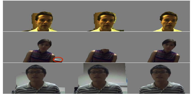
Figure 6. Comparison of segmentation results. The first column is obtained without contrast attenuation; the second column is the results using contrast attenuation based on the previous frame; the third column is obtained with contrast attenuation based on the previous frame and the temporal difference. We can see that contrast attenuation based only on the previous frame can produce false negatives (see the image at center).
