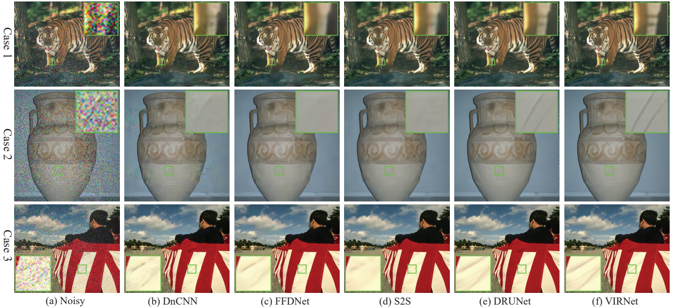
Fig. 4. Denoising results of different competing methods on three typical test examples of synthetic non-i.i.d. Gaussian Noise Removal.
