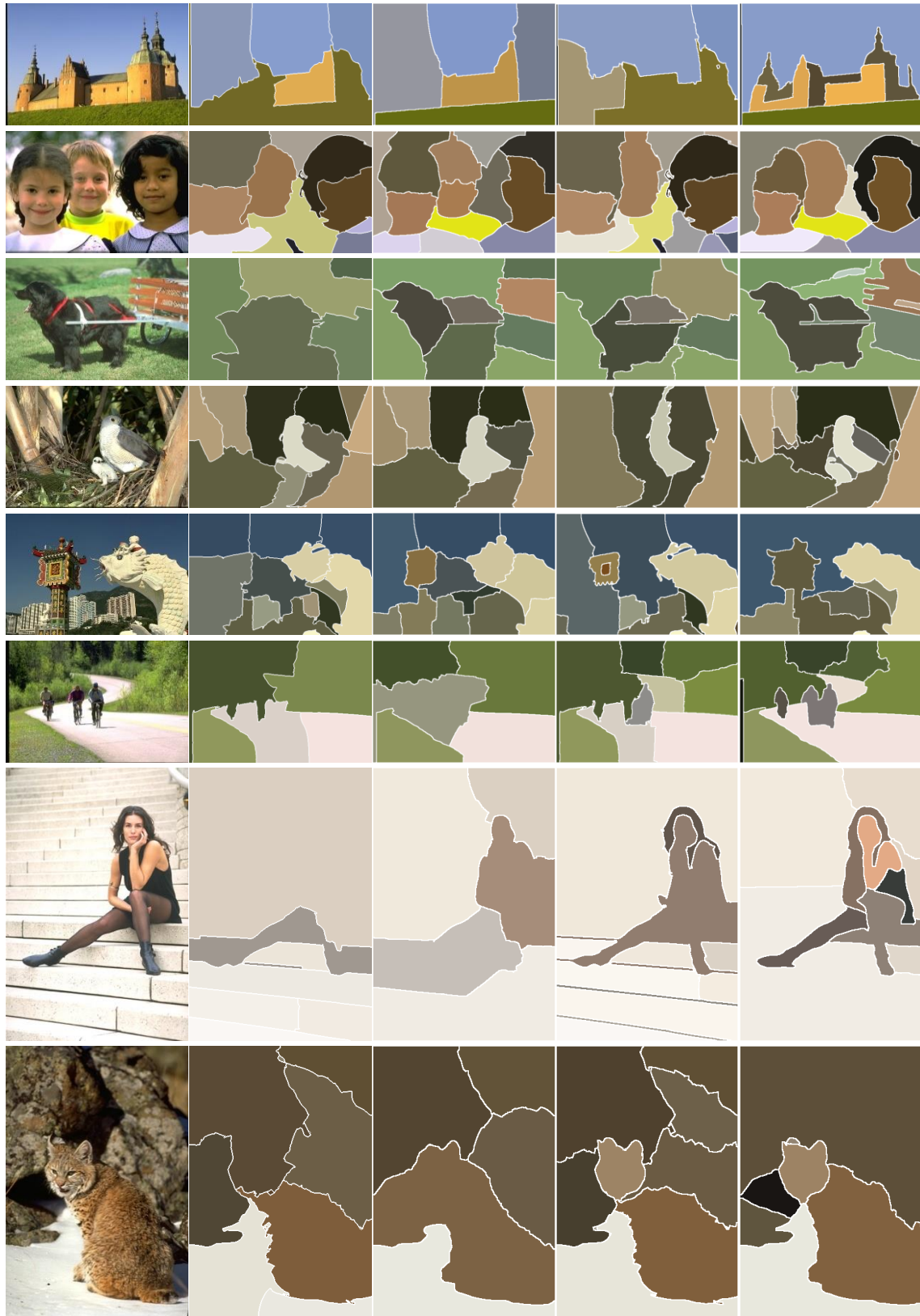
Figure 5. Comparison of segmentation results from NCut and clustering-based segmentation algorithms (Part II). From left to right: Input image; Normalized Cut; spectral clustering using mPb affinity; weighted spectral clustering using NCut affinity; revised clustering-based segmentation using our embedding with mPb affinity .
