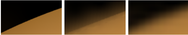
Figure 16: Magnification: original resolution \times 16 . Left: an accurate magnification by precise feature alignment. Middle: color bleeding caused by misalignment of vector representation to the feature. Right: bicubic interpolation.
