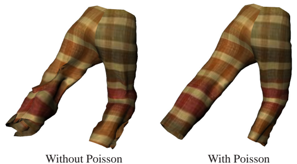
Figure 5: Deformation prediction without an additional translation solver may yield distorted results. However, once our Poisson-based translation solver has been applied, the resulting deformation becomes natural without artifacts.
