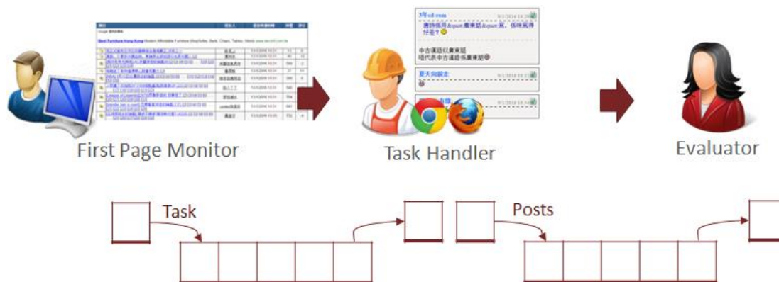
Figure 2: The system uses blocking queues to handle the interactions between classes
