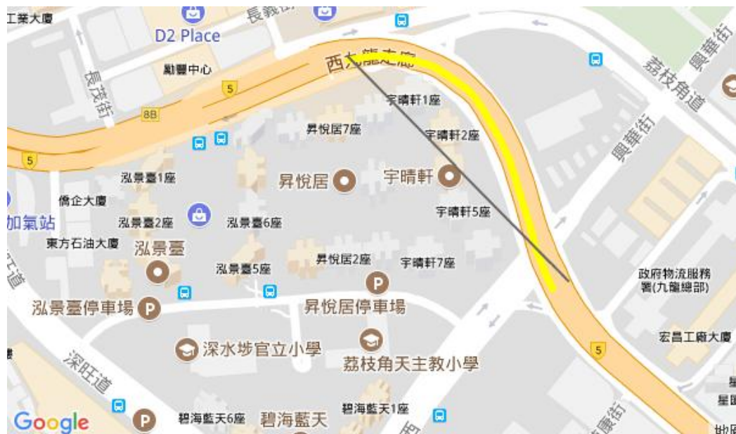
Figure 4 – Example of "Snap to road" function. The function returns the most likely roads (yellow line) according to the user input (black line).
