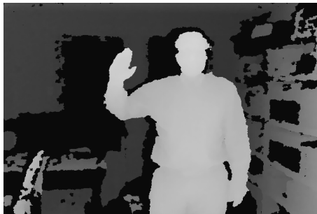
Figure 4.1: (Left) Kinect device. (Right) An example of noisy depth image obtained by Kinect.
