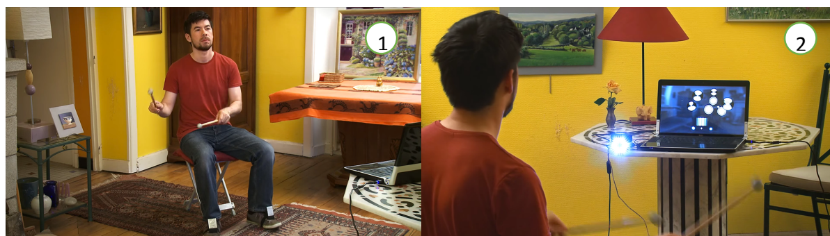
Figure 2: (1) Users hit the air to hit the invisible drums. (2) Users can see the position of the sticks to the drums in the computer. The glowing device is the lamp and camera.
