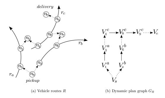
**Figure 3.2:** A collection of vehicles routes R, a dPDPT request  $(n_s, n_e)$  over R, and the dynamic plan graph  $G_R$ . The solid lines denote the vehicle routes/transport edges while the dashed lines denote the pickup, delivery and transfer with detour actions/edges.
