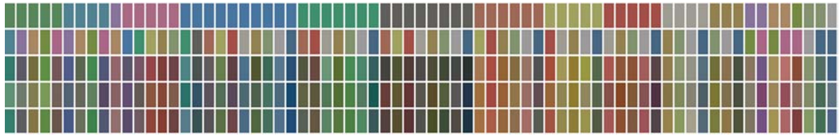
Figure 3: Pigment mixing using our neural network. The first and second rows are the two source pigments before mixing. The third row is the pigment mixing results sampled from real world experiment. The fourth row is the prediction of the pigment mixing behavior using our proposed neural network, but without employing the kernel functions. The fifth row is the prediction using our proposed neural network with the kernel functions.
