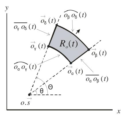
possible region  $R_{o}(t)$  is enclosed by four endpoints, two segments, and two arcs
