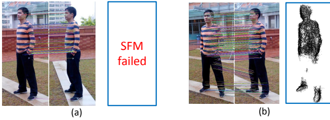
Fig. 2: Comparison of point correspondences obtained using ASIFT and NRDC. (a) ASIFT feature matching result (all correspondences are shown). SFM fails on such sparse correspondences. (b) NRDC matching result (only 1% correspondences are shown). SFM can successfully reconstruct a dense point cloud from such dense correspondences.
