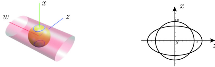
Fig. 2. Left: Intersection of the elliptic cylinder B' and the unit sphere A' ; right: the sectional view in the z - x plane.
