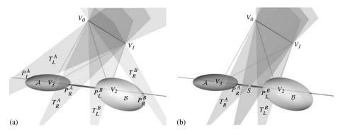
**Fig. 3.** (a) Four planes passing through  $V_0$  and  $V_1: \mathcal{T}_L^A$  and  $\mathcal{T}_R^A$  are tangent to ellipsoid  $\mathscr{A}; \mathcal{T}_L^B$  and  $\mathcal{T}_R^B$  are tangent to ellipsoid  $\mathscr{B};$  (b) A separating plane is one that passes through  $V_0, V_1$  and S, where S can be any point on the open line segment  $(P_R^A P_L^B)$
