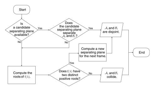
Fig. 4. Algorithm for collision detection between two ellipsoids  $\mathcal{A}_i$  and  $\mathcal{B}_i$  at frame i
