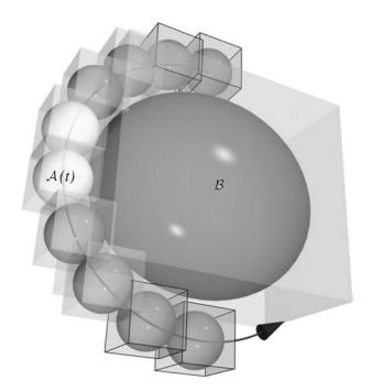
**Fig. 5.** Experimental set-up corresponding to the results in Table 2: a sphere  $\mathscr{A}(t)$  moves along a circular orbit around an ellipsoid  $\mathscr{B}$ . Bright spheres indicate collision. Framed boxes bounding  $\mathscr{A}(t)$  are disjoint from the bounding box of  $\mathscr{B}$
