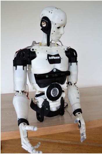
Figure 1: InMoov 3D life-size robot
