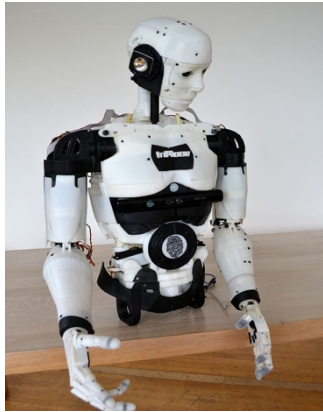
Figure 1: InMoov 3D printed life-size robot
