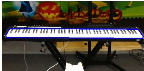
Figure 9: One remaining contour in quadrangle shape after filtering and approximation
