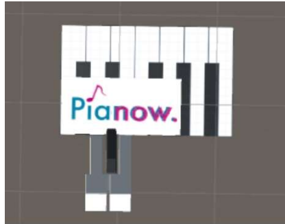
Figure 15: Image target setup with attached 3D keys that can be matched to an octave on the piano keyboard
