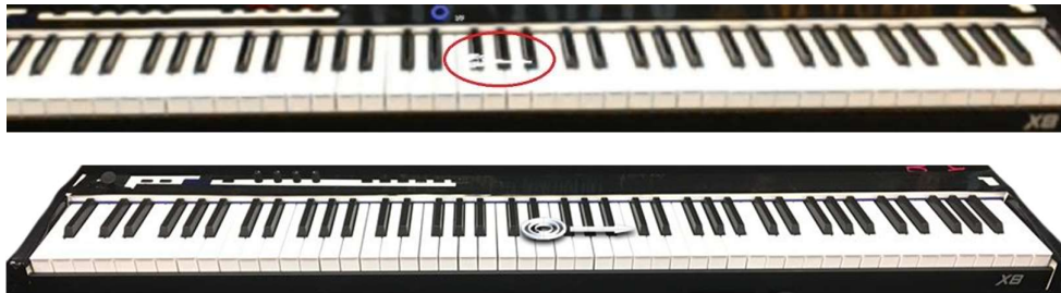
Figure 18: Indicator of the center of mass (the circle) and the orientation of the keyboard (the arrow) recognized by OpenCV
