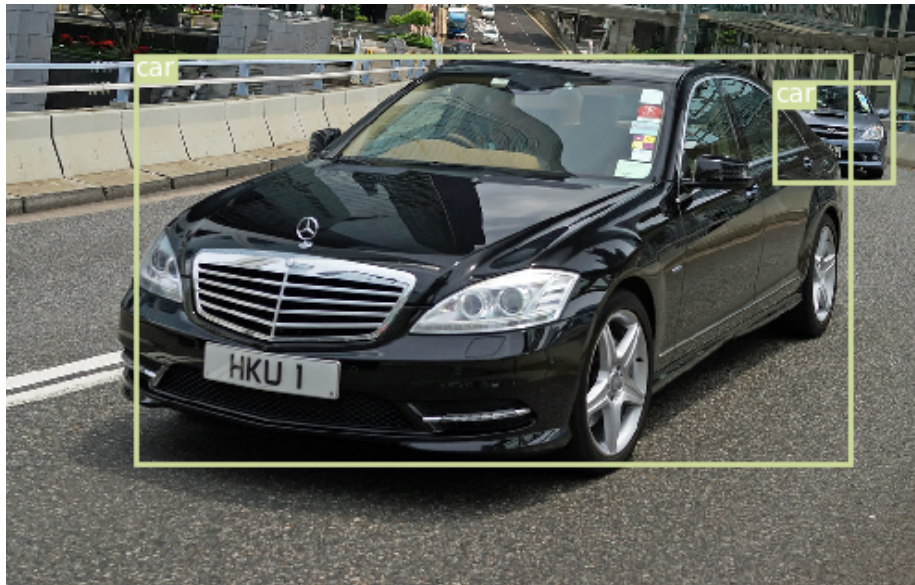
Figure 4.1: YOLOv3 Results. It shows two correctly identified cars and their location in image.
