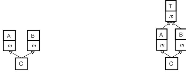
Figure 5.7: Fork inheritance (left) and diamond inheritance (right) on abstract methods.
