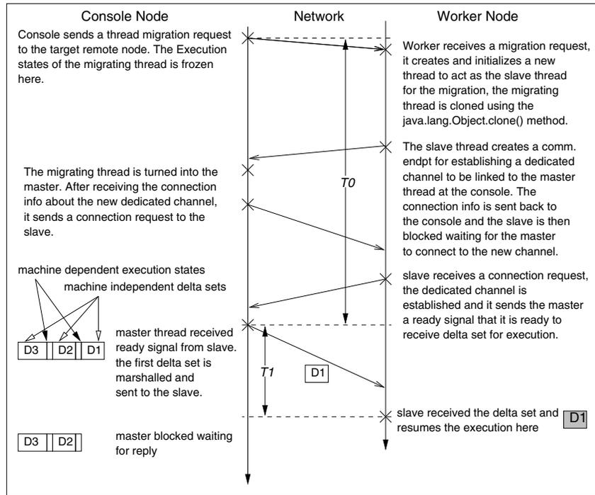
Figure 12: Interactions between the console and the worker during migration
