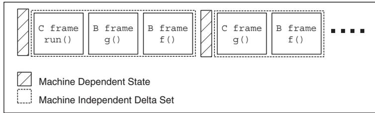
Figure 15: Execution Context of an instance of `DeltaE` Thread
