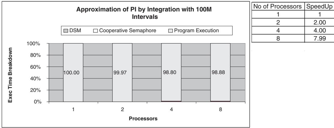
Figure 6: Performance results of the approximation of the value  $\pi$  with 100M intervals
