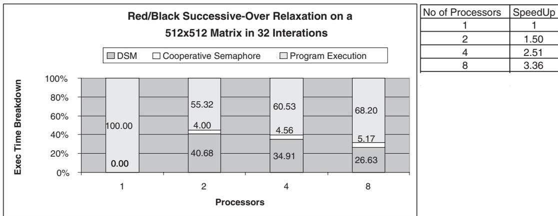
Figure 8: Performance results of the red/black successive-over-relaxation application on a 512x512 matrix
