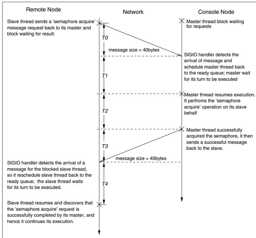
Figure 11: Cooperative semaphore in action: a migrated thread performs an acquire operation
