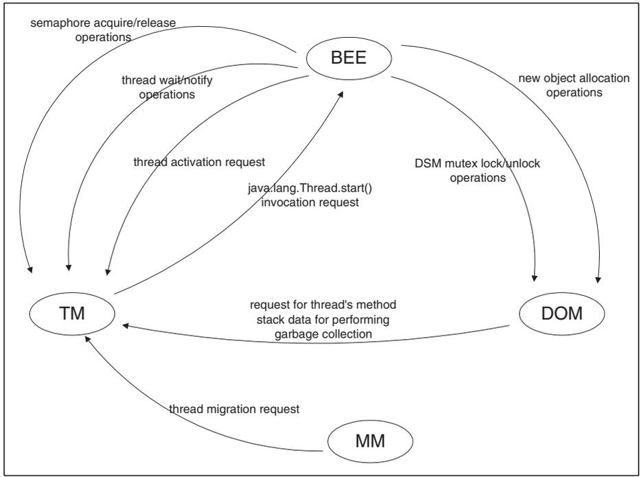
Figure 3: Interactions between system components in JESSICA
