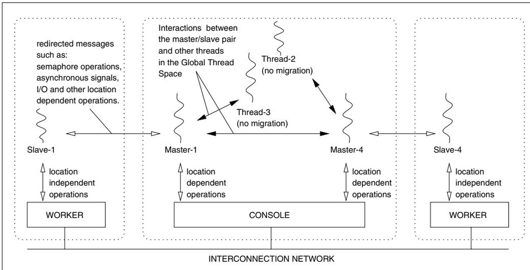
Figure 5: Interactions between the master and the slave threads that hide migration from the rest of the system
