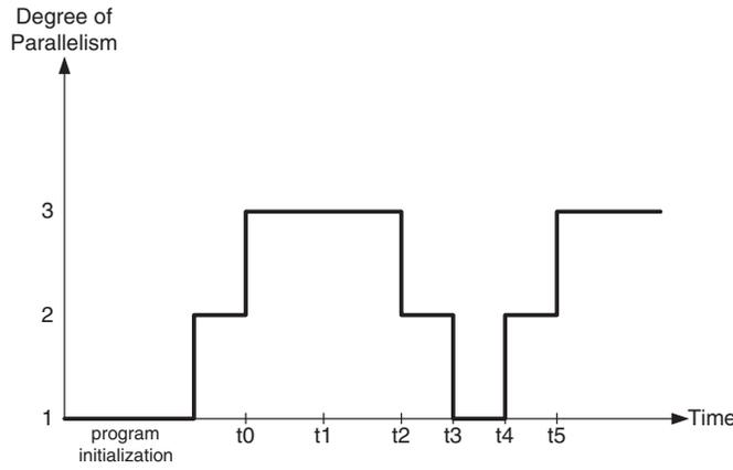
Figure 9: Change in Degree of Parallelism Against Time in the Dynamic Load Balancing Experiment
