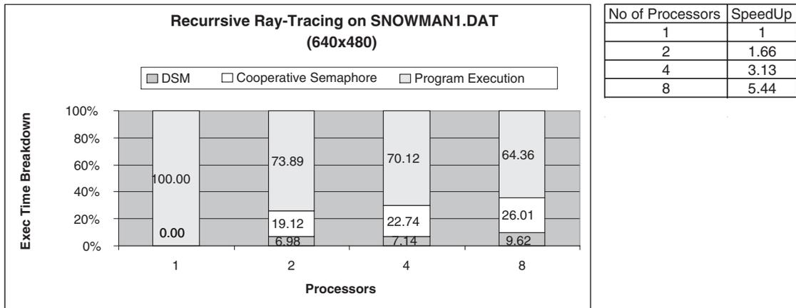
Figure 7: Performance results of the recursive ray-tracer to produce a 480x640 image
