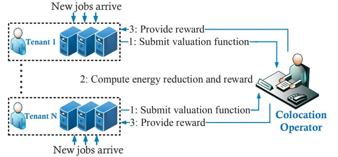
Fig. 2. An illustration of colocation EDR.
