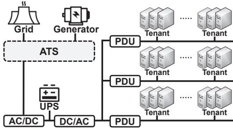
Fig. 1. Power Architecture in a Multi-tenant Data Center
