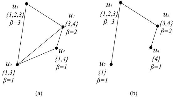
Fig. 1. a) The potential graph: the set besides each SU is its available channels, and  $\beta$  its number of antennae. Two nodes do not have an edge (e.g.,  $u_1$  and  $u_4$ ) because their distance exceeds at least one of their transmission ranges. b) The realization graph which is connected: the set besides each SU is the channels assigned to it.
