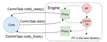
**Figure 6.** Interaction between Core and framework engines without global barrier, *e.g.*, MXNet. Only one DNN layer is shown (assume one tensor in the layer). Operations in squares are added by ByteScheduler. The solid arrows are direct function calls, while the dashed arrows mean dependencies.
