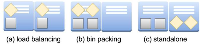
Fig. 3. Placement under different schemes (diamonds represent parameter server and worker in job 1; squares represent those of job 2).
