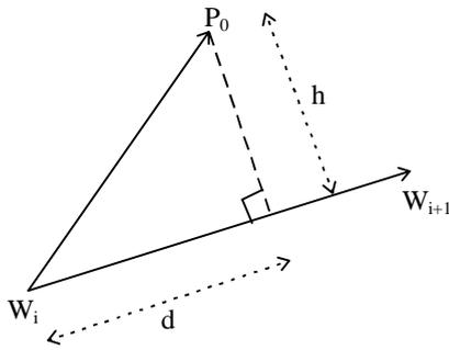
Figure 3: Calculations involved in Interpolation
