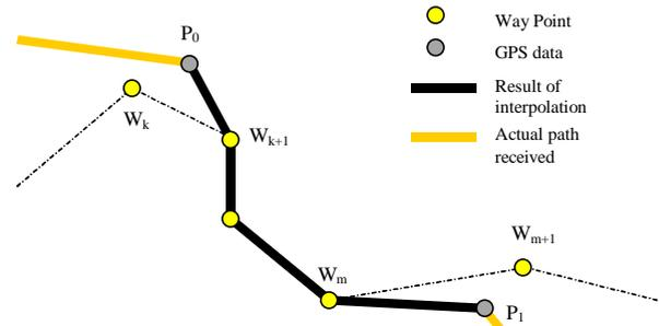
Figure 2: Interpolation of GPS data
