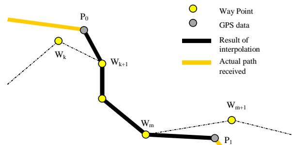
Figure 2: Interpolation of GPS data
