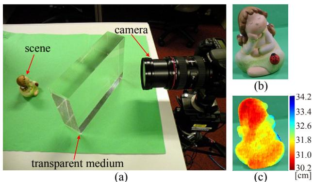
**Fig. 1** (a) Experimental setup. (b) A direct image of the scene. (c) A reconstructed depth map of the scene.
