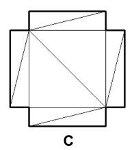
In the examples, the heavy line is the outline of the polygon and the lighter lines give the *triangulation*. In each case a triangulation of a polygon with n vertices will result in (n-2) triangles.
