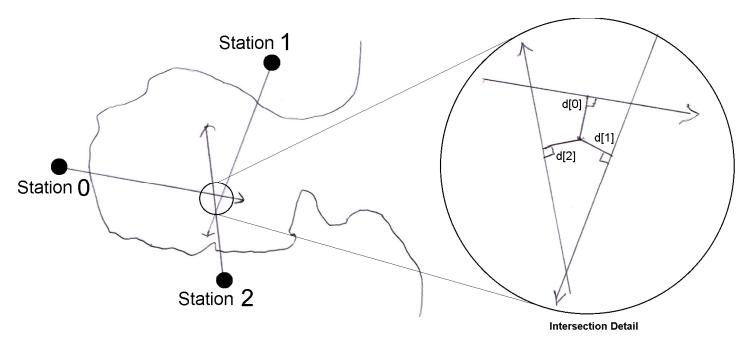
Station 1 is 3.715 kilometers east and 1.765 kilometers north of station 0 and station 2 is 2.894 kilometers east and 2.115 kilometers south of station 0.
