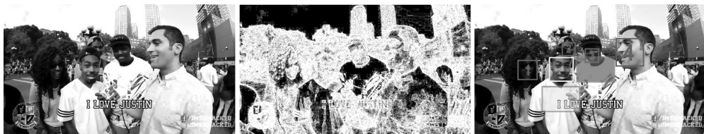
Fig. 12. Use of saliency map in a complex background. Left: original screenshot; Middle: a saliency map used in the method of Hong et al. [2010]; Right: subtitle placement by our method (yellow shadowed rectangle) vs. that by Hong et al. [2010] (green shadowed rectangle) for the speaker (yellow rectangle), red rectangles are nonspeakers. The subtitle placement by the method of Hong et al. [2010] mistakes the nonspeaker #4 to be speaking and blocks nonspeaker #3, thus confusing the viewer. Screenshots with permission from YouTube video v=tpBtdKRDVbI .
